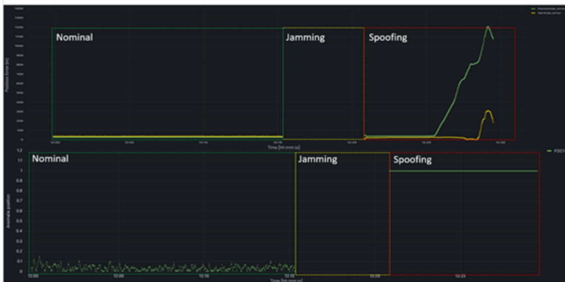
Figure 3 – Analysis of Vertical and Horizontal Position Errors and the corresponding position anomaly indicator based on the analysis of position errors. The figures are divided in three different sections defined by the presence of three different boxes (green, yellow, red). These sections correspond to nominal case without interferences (green), strong jamming attack (yellow) followed by a spoofing attack (red)
