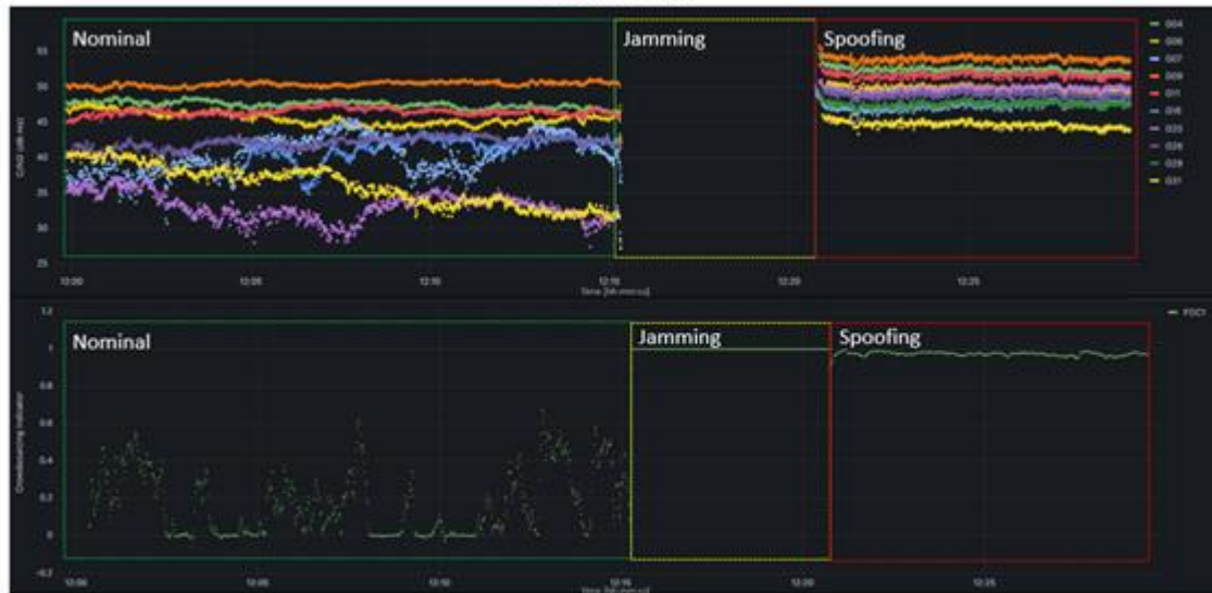
Figure 3 – Analysis of CNO measurements and the corresponding crowdsourcing anomaly indicator based on the analysis of CNO measurements. The figures are divided in three different sections defined by the presence of three different boxes (green, yellow, red). These sections correspond to nominal case without interferences (green), strong jamming attack (yellow) followed by a spoofing attack (red)
