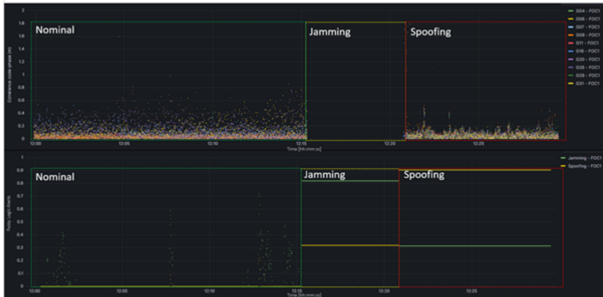
Figure 4 – Analysis of code-phase coherent anomaly variation and the Fuzzy Logic Output Alerts (Aggregation of all Anomaly Event Indicators), notably Jamming and Spoofing Alerts. The figures are divided in three different sections defined by the presence of three different boxes (green, yellow, red). These sections correspond to nominal case without interferences (green), strong jamming attack (yellow) followed by a spoofing attack (red)
