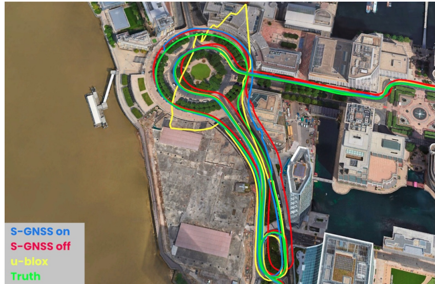
Figure 7. Case 2: Multiple roundabouts, including a tunnel, with high-rise buildings to North and East. Green is the GTS, yellow is the u-blox mass market receiver, red is the SDR with S-GNSS switched off, and blue is the SDR with S-GNSS switched on.
