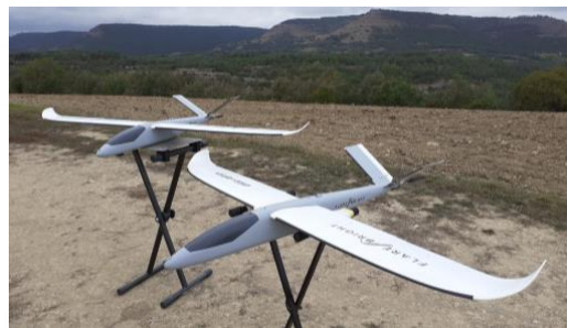
Figure 1. The two CATUAV ATMOS-8 platforms used as flight test demonstrators for this work.
